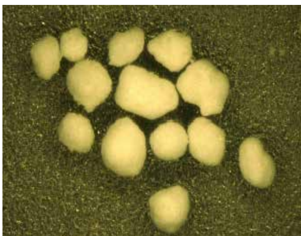
Figure 4: Lactose granules (light microscope, magnification: 50x)
