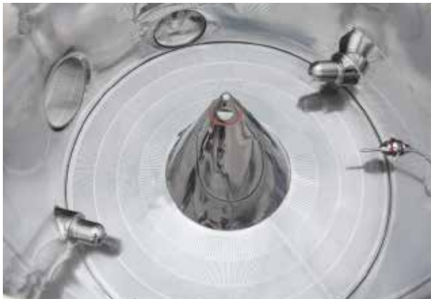
Figure 2: Bohle Uni Cone BUC® with tangentially mounted spray nozzles within a BFS 30
