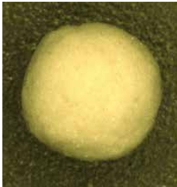
Figure 5: Single spherical lactose agglomerate (light microscope, magnification: 50x)
